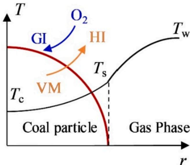
Fig. 2. The physical model for ignition of single coal particle with intraparticle temperature gradient (GI: Heterogeneous ignition, HI: Homogeneous ignition).
