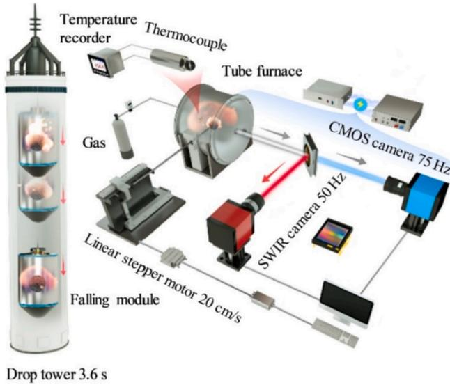
**Fig. 3.** The scheme of the microgravity experimental system.
