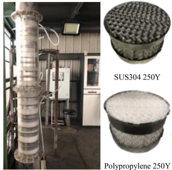
Fig. 3. Testing hydrophilic modified polypropylene structured packing.
