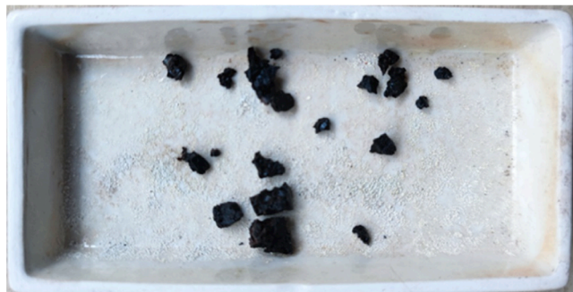
Fig. 17. The slag fragments in the muffle furnace during the thermal cycle test.
