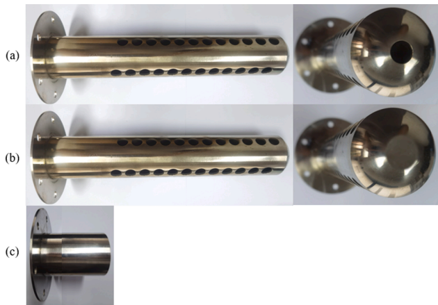
Fig. 3. Different types of jet mixing.
