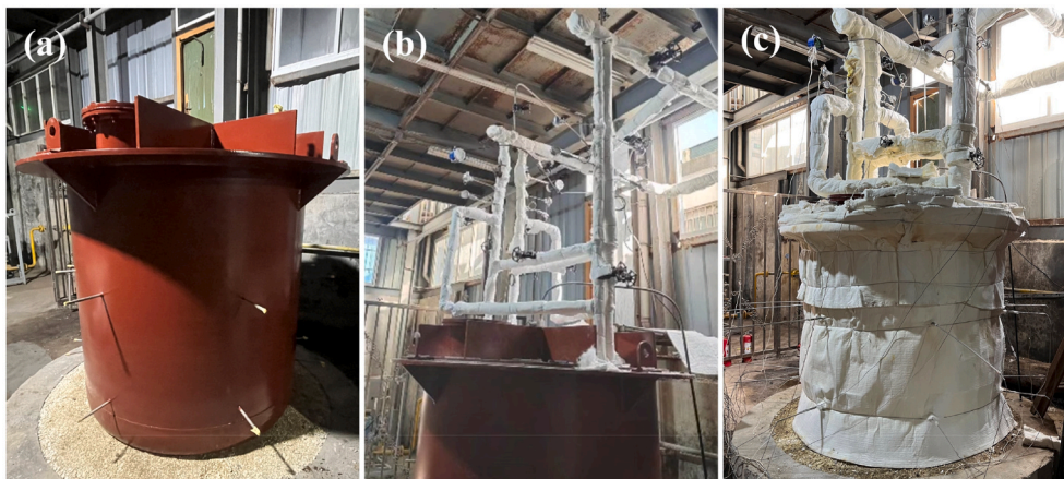
Fig. 2. Photographs of the PCM tank: (a) without tube connection, (b) with tube connection, and (c) with tube connection and aerogel insulation.
