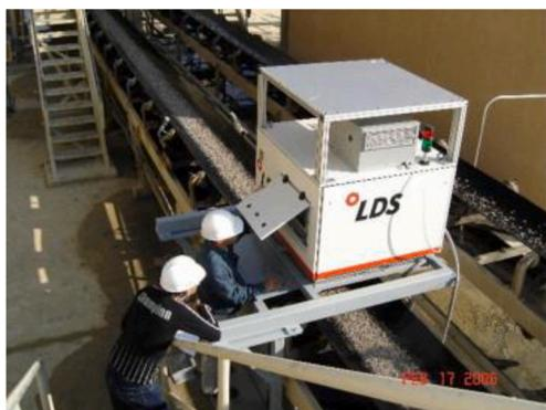
Fig. 5. Online LIBS system (LDS) on a moving belt conveyor developed by Gaft et al. [60].
