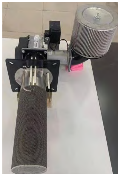
Fig. 2 Physical diagram of the metal fiber surface burner
