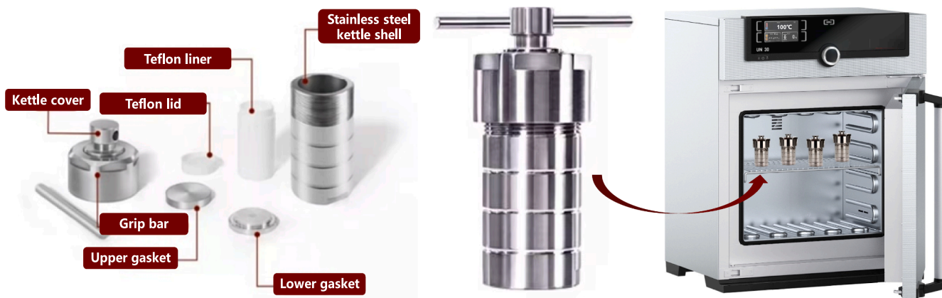
Fig. 3. Hydrothermal synthesis autoclave and oven for immersion corrosion experiment.
