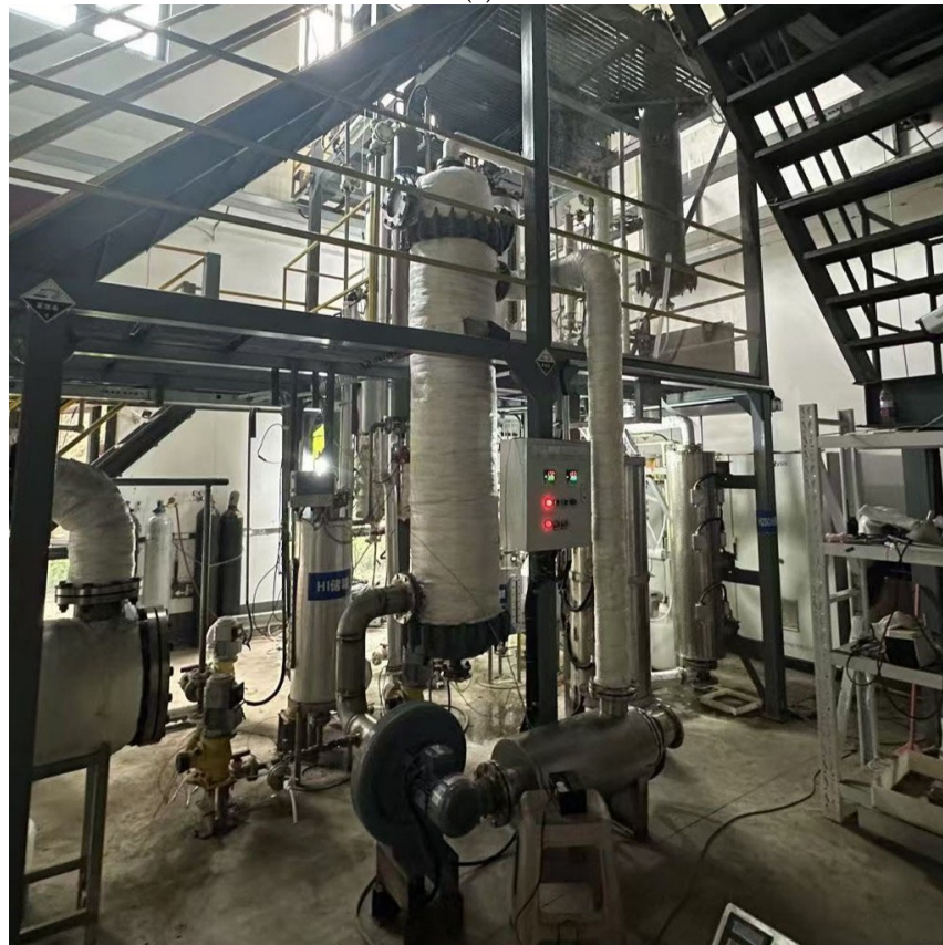
Figure 3. H_2SO_4 evaporator: (a) conceptual images; (b) physical images.
